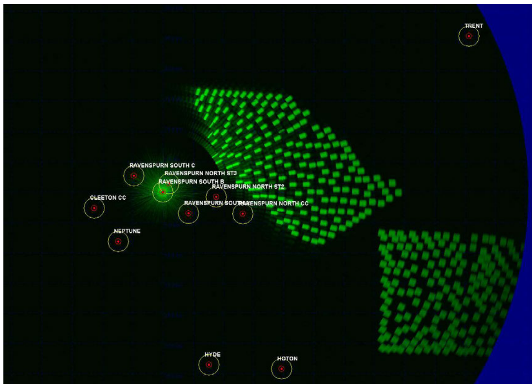
Figure 24: Ravenspurn South B platform REWS detection threshold over the cumulative Hornsea Projects array area.
